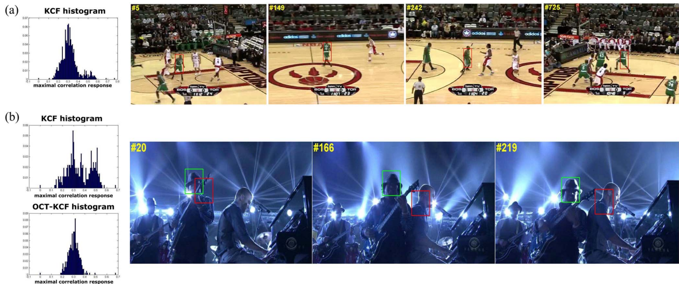
Fig. 6. Illustration of KCF and OCT-KCF on Basketball and Shaking sequences. (a) Good performance is achieved when the response (output) of KCF is observed to follow a Gaussian distribution on the Basketball sequence. (b) OCT (green rectangular) is used to improve the performance of KCF (red rectangular) on the Shaking sequence, and correlation response in OCT-KCF follows a Gaussian distribution.
