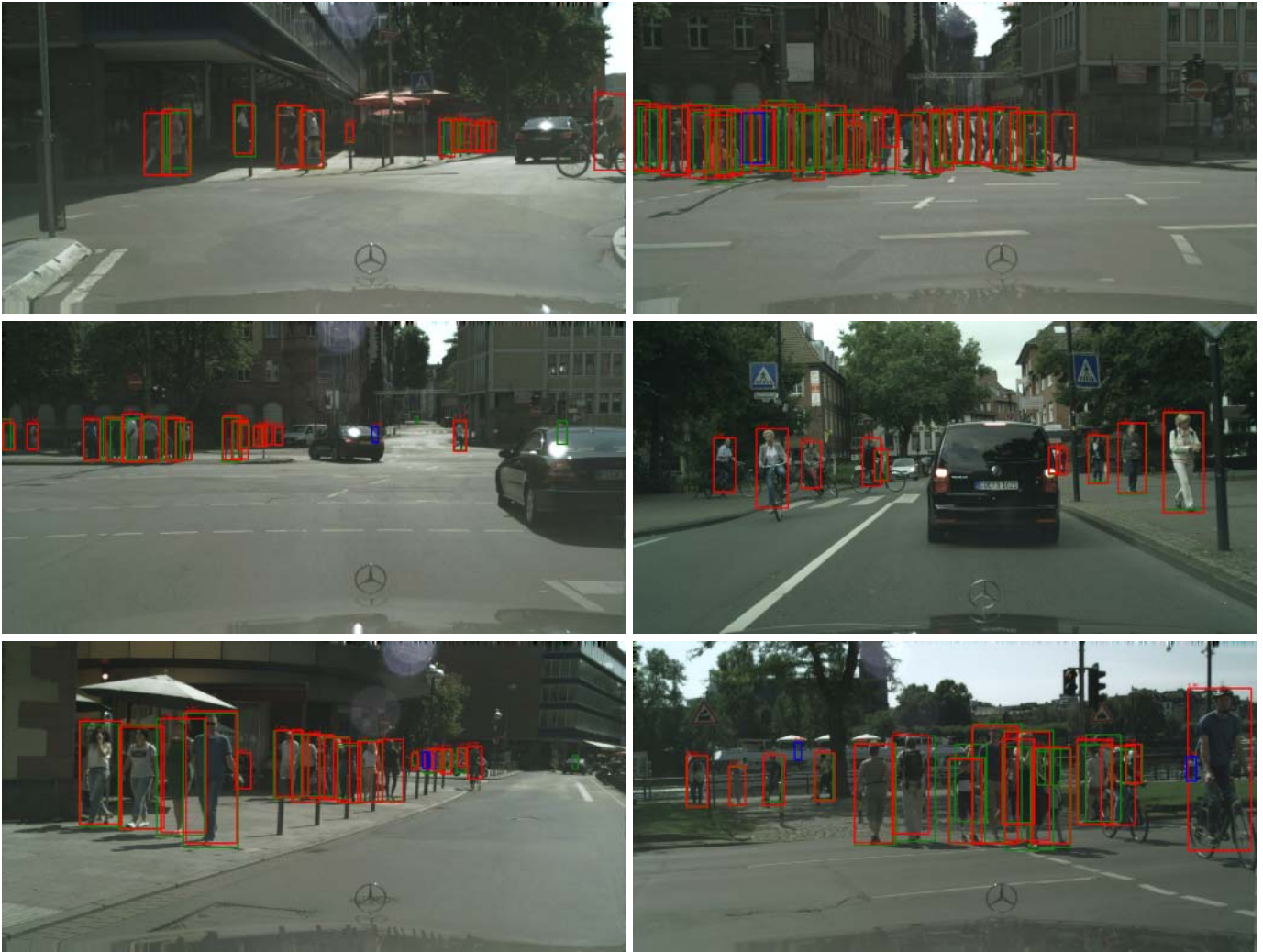
Fig. 11. Examples on the CityPersons. The red, blue and green boxes indicate correctly detected pedestrians, false positives, and ground-truth, respectively.
