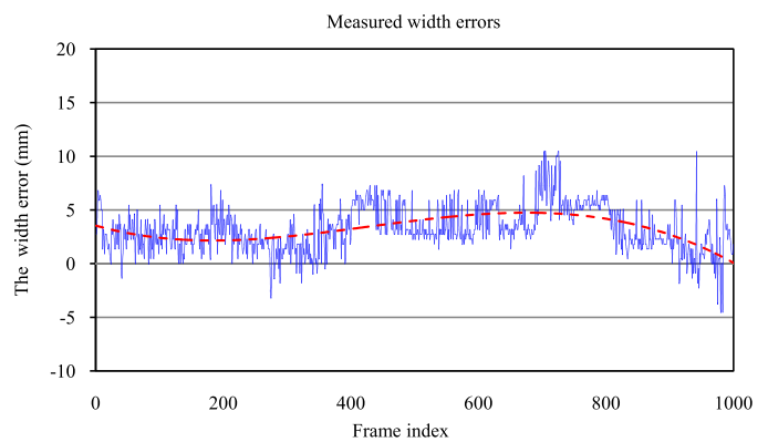
Fig. 17. Weld width measurement errors by the STC-HMMs. It can be observed that there are abrupt large errors in some frames. The errors reduce much after several frames.
