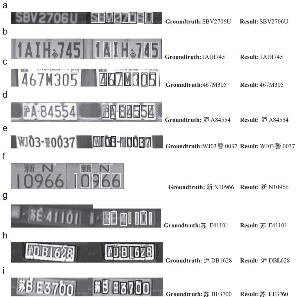
Fig. 11. Segmentation and recognition examples (with failure examples).
