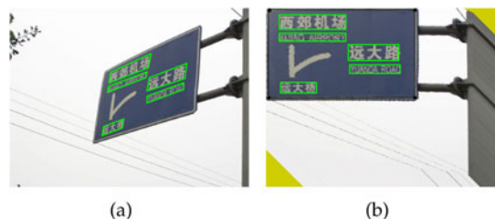
Fig. 11. Perspective correction of text with a homography operation [65]. (a) Text of perspective distortion. (b) Corrected text.
