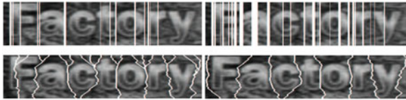
Fig. 8. Character segmentation with the projection profile analysis (first row) and the path optimization method (second row) [139] (Courtesy of Phan).
