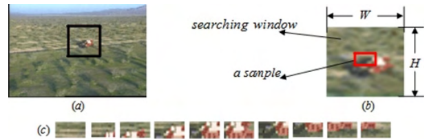
Fig. 2. (a) The searching window of the object. (b) A sample. (c) Examples in the sample set.
