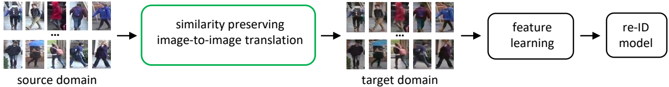
Figure 2: Pipeline of the “learning via translation” framework. First, we translate the labeled images from a source domain to a target domain in an unsupervised manner. Second, we train re-ID models with the translated images using supervised feature learning methods. The major contribution consists in the first step, i.e. , similarity preserving image-image translation.
