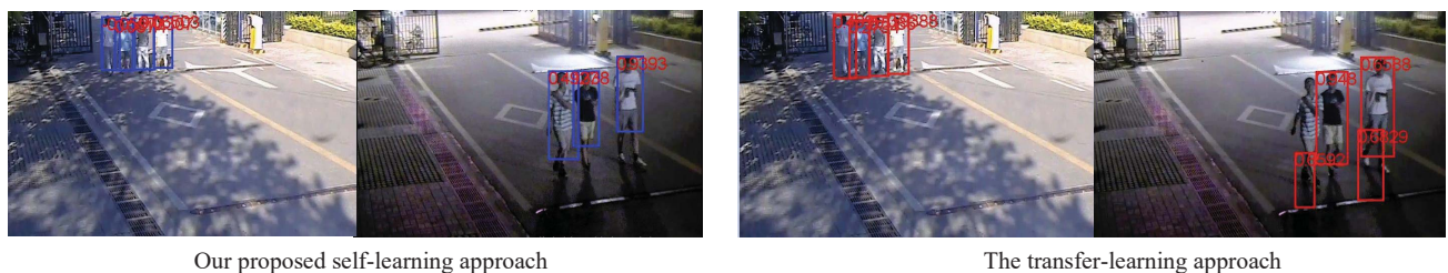
Figure 8. Detection results on 24Hours dataset. The self-learning detection correctly detects all pedestrians from the daytime (left) and night (right), but transfer learning has missed and false detections.
