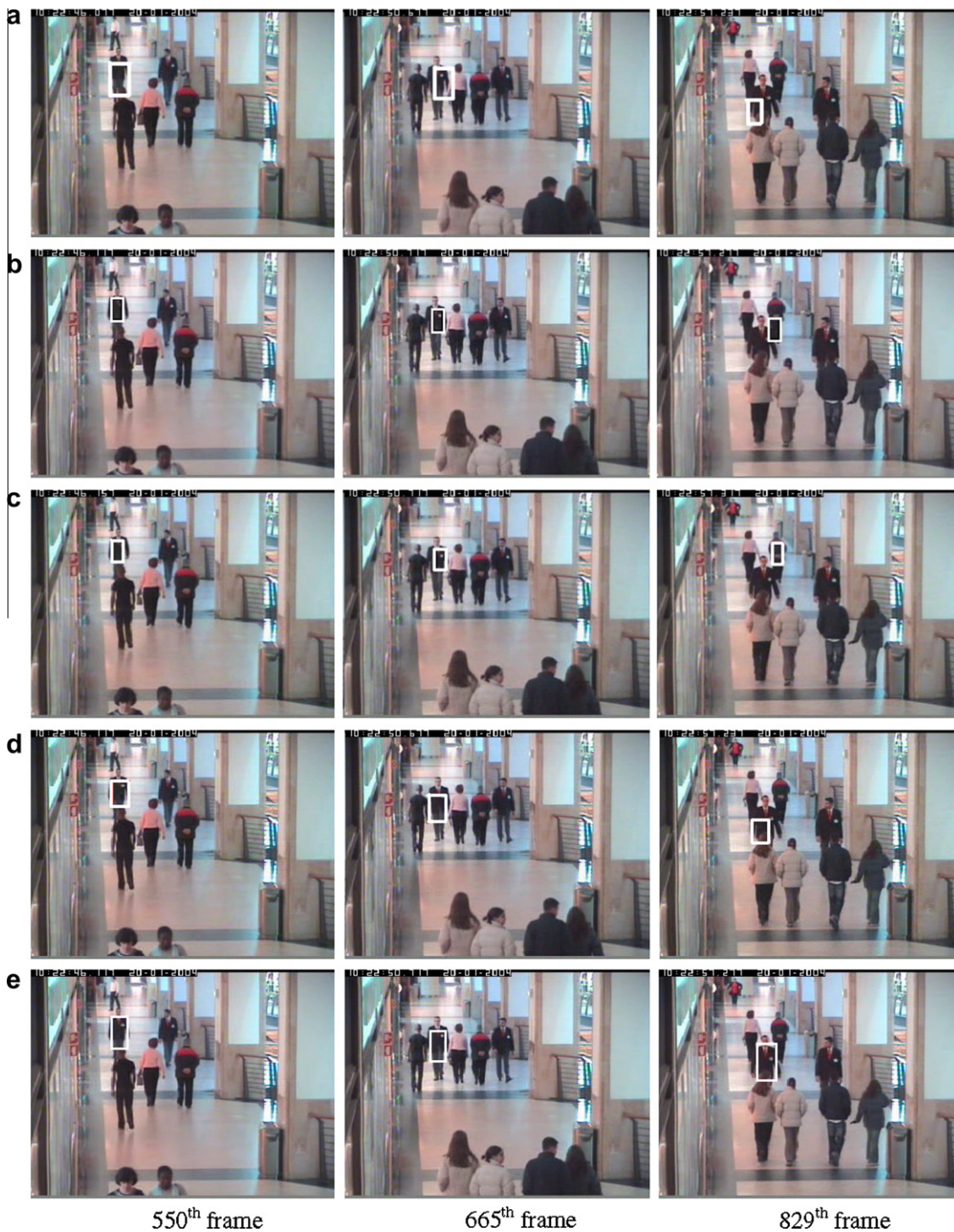
Fig. 10. Tracking results of some occlusions and scale variation. (a) Results of color-based tracking method. (b) Results of variance ratio feature shift method. (c) Results of Peak difference feature shift method. (d) Results of our proposed tracking approaches based on HOGC feature evaluation in Kalman filter and (e) in Particle filter.
