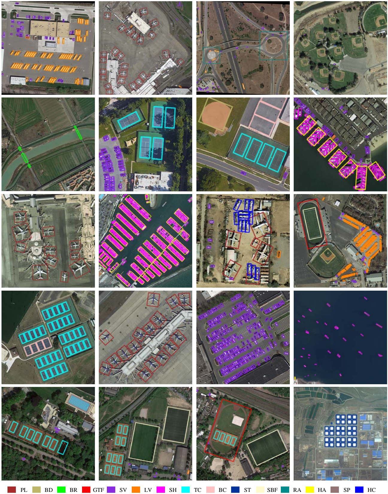
Figure 7: Qualitative detection results on the DOTA-v1.0 dataset. Category labels are the same as in Table 4.
